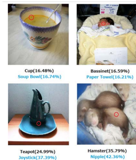
Fig. 16: Examples of one-pixel-attacks on the Imagenet database, borrowed from [65]. These represent contrastive singletons .
