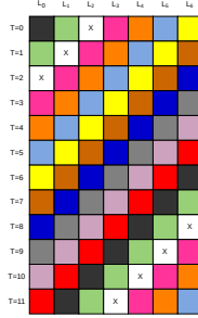
Fig. 9: A visual scheme of the “sliding window” constraints for encoding a 12-step full cycle. In the case of encoding a RIGHT CYCLE , the constraints should be read from top to bottom. In the case of encoding a LEFT CYCLE , the constraints should be read from bottom to top.
